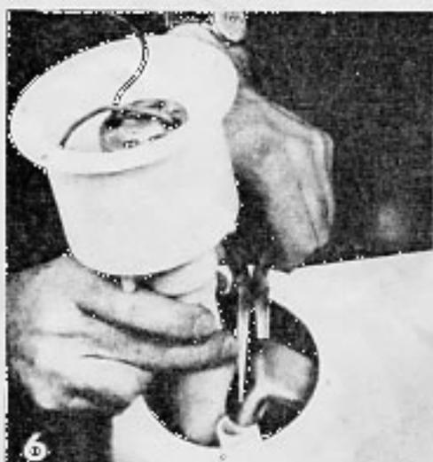
6 Bend hose as shown and push fit  $\frac{1}{2}$  to  $\frac{3}{4}$ " onto hose nipple of cartridge, make sure red mark on hose and cartridge line up. Use vaseline or glycerin around inside of hose to facilitate insertion.
