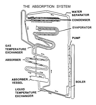
The cooling unit parts that accomplish this 'cooling' or heat extraction process, include the:
