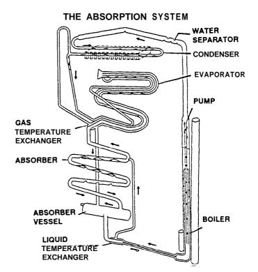
Before this cooling system can properly extract heat from the cabinet of the refrigerator, three requirements for proper refrigerator operation must be met. These are precise heat, specified ventilation and proper leveling.
