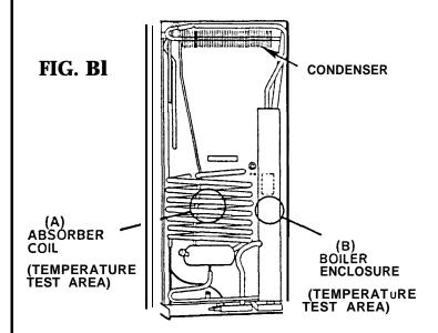
Under normal operation the temperature at the absorber coils (A) and the boiler (B) should be approximately the same. If the temperature at the absorber coils (A) is much hotter it indicates loss of refrigerant and the cooling unit must be replaced. If the temperature at the boiler (B) is very hot and the absorber coils (A) are cool it indicates that the refrigerant is not circulating properly. This could indicate:
